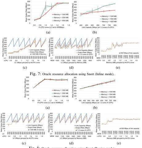
Fig. 8: Oracle resource allocation using Snort (Passive mode).
