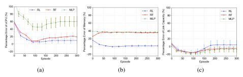
Fig. 12: Percentage error of resource allocation predictions by MLP, RF and RL regarding the vFW VNF.
