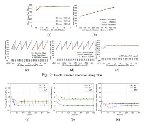
Fig. 10: Percentage error of resource allocation predictions by MLP, RF and RL regarding Snort (Inline mode).
