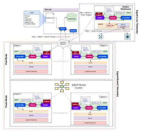
Fig. 3. System Level Diagram of the Telemetry System
