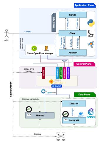
Fig. 4. iRaaS Deployment Diagram
