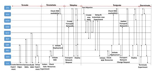
Fig. 4. 5G-VIOS workflows for creation, instantiation, deployment, migration, and termination of an experiment.
