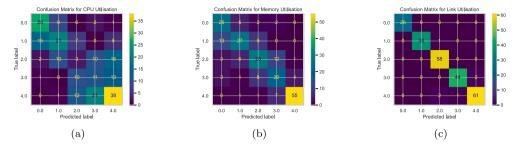
Fig. 7. Performance of the profile-based classification model based on the confusion matrices for predictions of (a) CPU, (b) Memory, and (c) Link resource utilisation.
