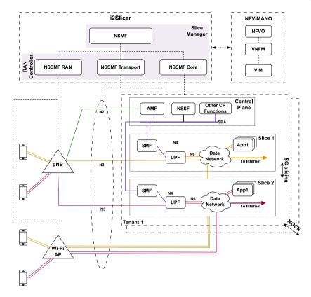
Fig. 5. i2Slicer: Multi-RAT network slicing architecture.
